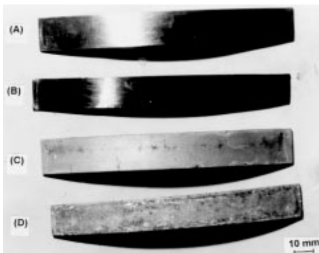
Fig. 4 Surface appearance of (a) type 304 stainless steel, (b) Zircaloy-2, (c) Al-1S (oxidized), and (d) Al-1S (polished) samples after exposure with CBB assemblies in spent fuel storage pool for 6 months
